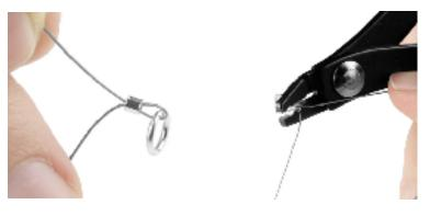
STEP 5: Next, squeeze the crimping pliers, bringing the dimple down in between the two wires so that the strands are trapped on opposite sides of the crimp. It is important that you don't have a death grip when you are crimping, because this will weaken the crimp. However, you do want to give it a good squeeze. You should now have a U-shaped crimp tube.
