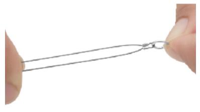
STEP 6: You will then move the crimp to the second station of the crimping pliers, placing it so that when you squeeze, the two sides of the U will come together. Give it a nice squeeze. With the nipper tool, cut the excess wire.
