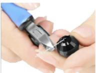
STEP 3: Position your round nose pliers at the end of the tail, making sure the tail faces away from your body. Wrap the wire towards you to create a loop.
